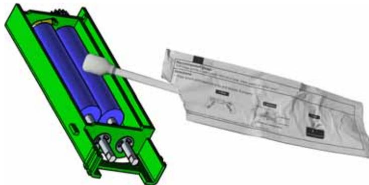
When finished using the cleaning swab to clean the rollers, rinse the rollers under running water again to remove any traces of isopropanol left by the swab. Allow the rollers to dry completely before reinstalling the cleaning unit.
